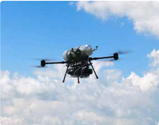
ZAL's LH 2 drone during its successful maiden flight in July 2026. Clearly visible: the cylindrical liquid hydrogen tank.
